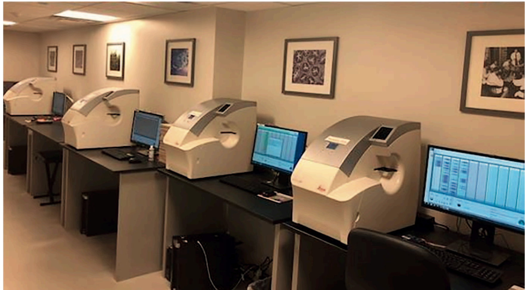
Figure 1. Digital pathology suite. Whole slide scanners and computers are arranged ergonomically for digital pathology supervisors and technicians to manage scanning workflow.
